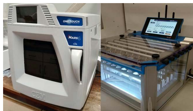
Fig 1.2. Microwave digestors and nitrogen evaporation systems.
