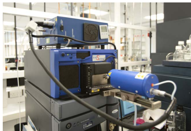
Fig 2.3. DART-QDa system for screening of animal feed extracts for mycotoxins.
