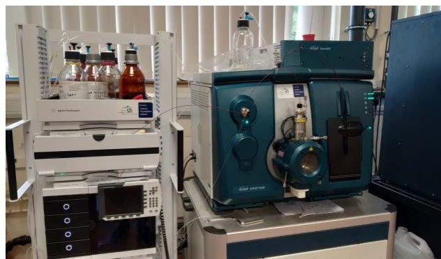
Fig 1.1. 6500+ Qtrap MS system for targeted analysis.
