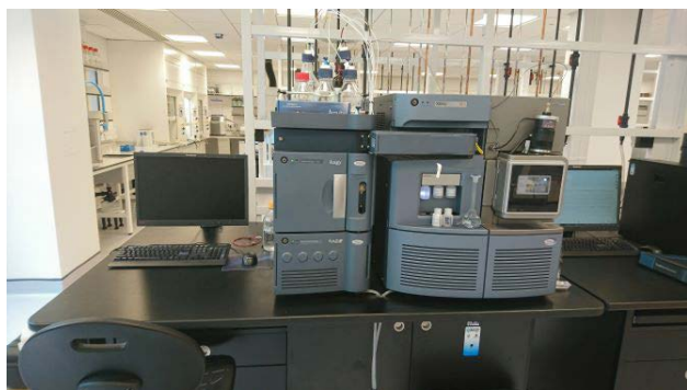
Fig 2.1. Waters Xevo TQ-S coupled to an Acquity i-class LC system for targeted analysis.
